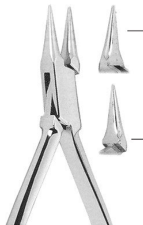
3235 Double rounded jaw wire bending pliers. For wires up to 0,7 mm. (.028").
